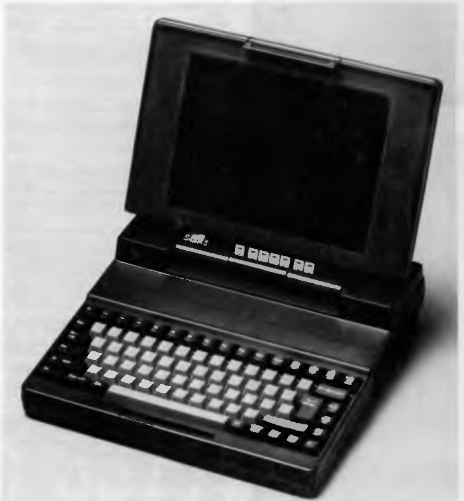
Figure 2. The Super 5 has a screen resolution of 600 x 400, a quick 20 megabyte disk and an 80286 processor — just right for laptop publishing!
