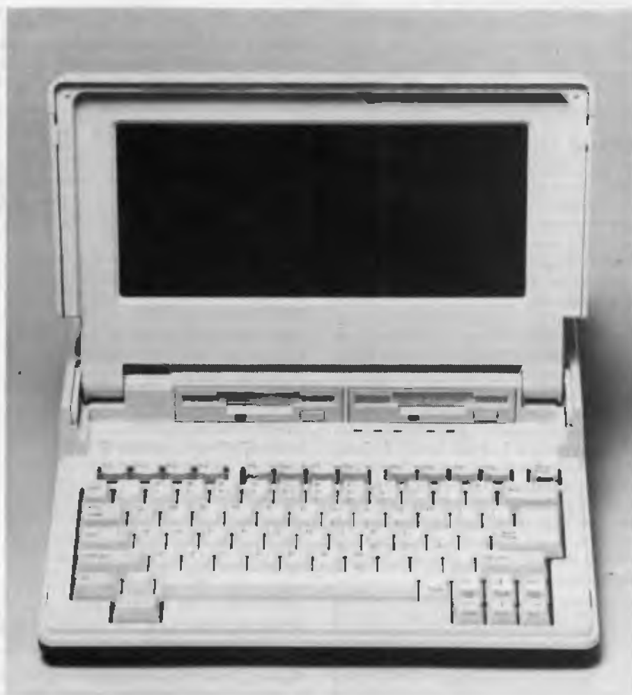
Figure 1. The Tandy 1400LT has a superb blue and white (monochrome) screen and comes with 768 Kbyte of RAM as standard. Note the convenient position of the disk drives.
