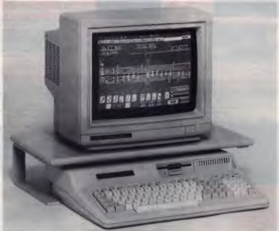
Figure 3. The standard 1000 HX, with the keyboard attached to the system unit, has one disk drive and MS-DOS commands in ROM.
