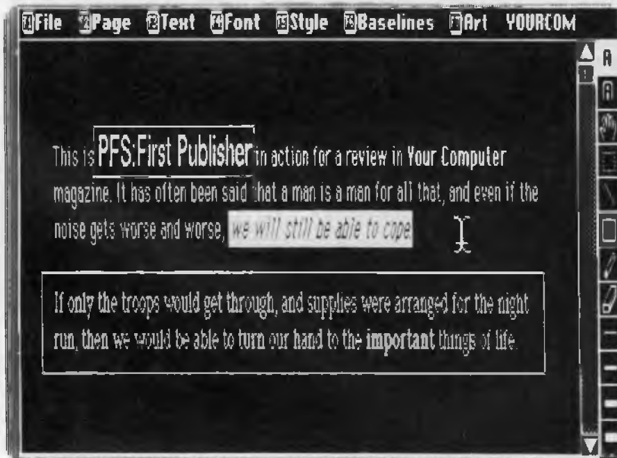
Figure 4. It's easy to put rectangular borders around words or paragraphs with PFS:First Publisher; the words 'we will still be able to cope' are highlighted in preparation for changing the font or style.
