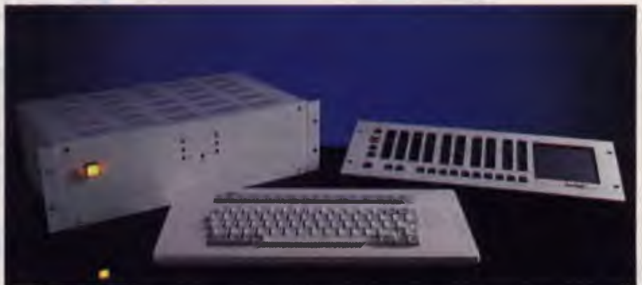
Figure 3. For video and media work, one of the machines recommended by the Victorian Department of Education is the Fairlight CVI (Computer Video Instrument) – this is the educational model mentioned in the text.
